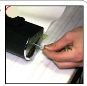
with a firm, secure hold on the graphic, remove the graphic roller pin
