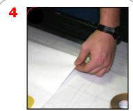
attach the bottom of the graphic to the leader strip (back of graphic attaches to leader strip)
