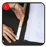
Remove paper backing from the tape on the graphic rail.
